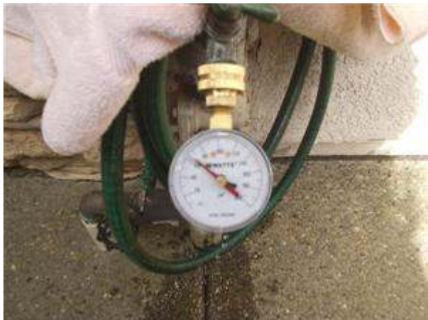
4.0 Picture 1 water pressure at 62 lbs
